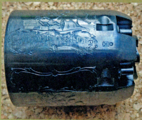
(Above) U.S.M.R. marking on the cylinder, note the proof marks could be better placed. (Left) Detail of the safety pins and ratchet on the rear of the cylinder
