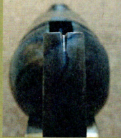
Detail of the rear sight cut into the hammer
