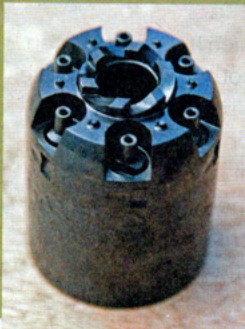
(Above) U.S.M.R. marking on the cylinder, note the proof marks could be better placed. (Left) Detail of the safety pins and ratchet on the rear of the cylinder
