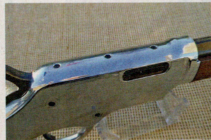
The receiver is drilled and tapped for a scope rail
