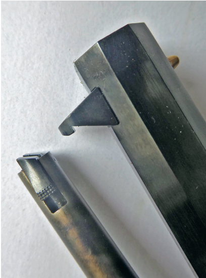
The loading lever locking arrangement is very secure, note the octagonal barrel
