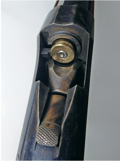
The cartridges are extracted rather than ejected
