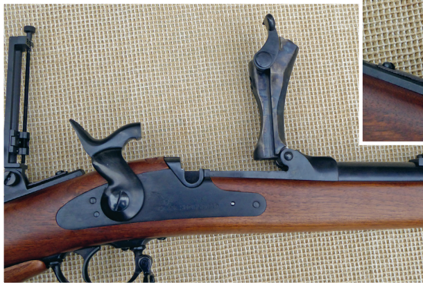
(Above) Detail of the vertical graduations on the Creedmoor rear sight (Left) Hammer on half cock with trapdoor wide open
