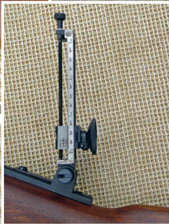
(Above) Detail of the vertical graduations on the Creedmoor rear sight (Left) Hammer on half cock with trapdoor wide open
