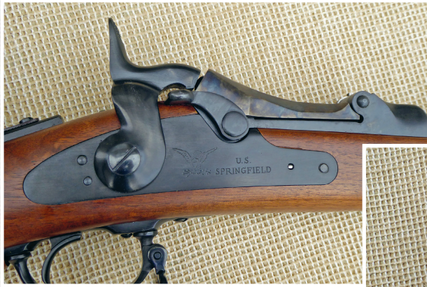
(Left) Percussion-era lock plate and hammer. The trapdoor opening spur is just under the hammer nose
