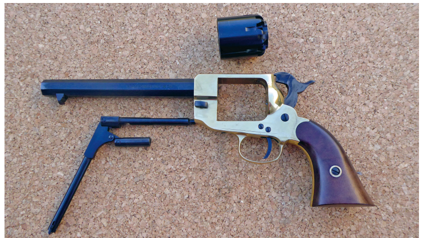
Stripped showing rammer system, arbour pin and cylinder. Closed-framed revolvers are stronger than the Colt, open-frame types
