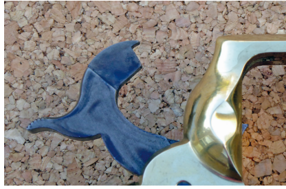
Small capping cut-out and Remington-style hammer
