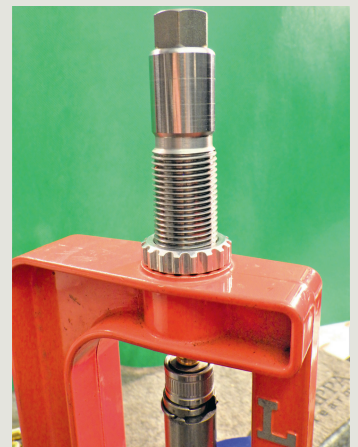
The die holds the case while the primer pocket is swaged
