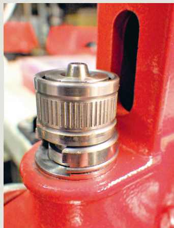
The swage holder takes the place of a shell holder on the ram and reforms the primer pocket to remove the crimp
