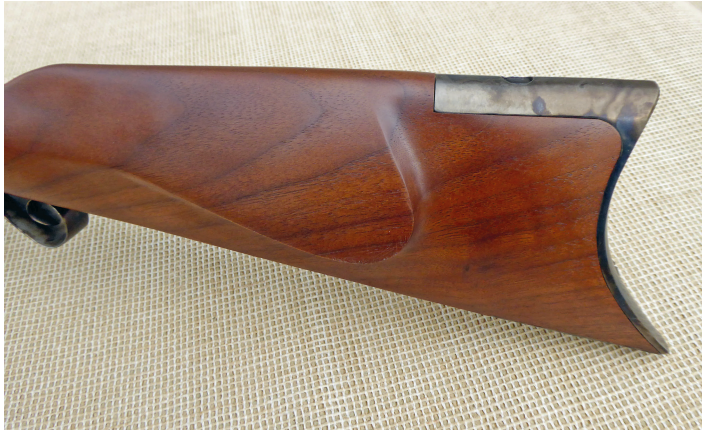
Detail of the cheekpiece, note minor gaps in the wood-to-metal fit
