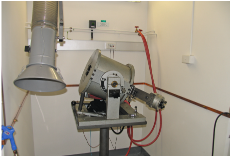
If you have room on your reloading bench, a closed bomb is the device you need for measuring powder burn rates
