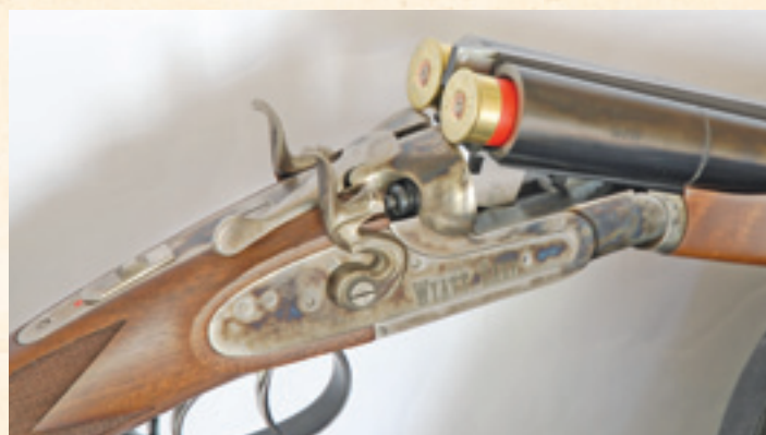
The Wyatt Earp shows rebound hammers and a separate safety catch, typically it's a non-ejector. The front trigger fires the right barrel and the rear the left
