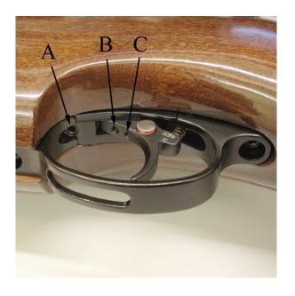
This rifle is fitted with a manual safety button located in the trigger blade. To make the rifle safe the button must be pressed until it is flush with the side of the trigger blade.
