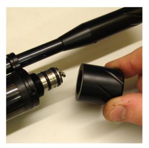
Once the connector is exposed the female part of the filling kit can be place on the male and press all the way on making sure that the 'O' rings on the male part are covered.
