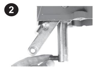
Install new stepped Ram Pin into ram
