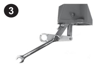
Install toggles and tighten using 9/16" wrench. Tighten to allow free movement, without side-to side-play.
