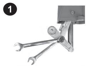
Remove existing handle, toggles and ram pin. Use 9/16" wrench to remove link bolt.
