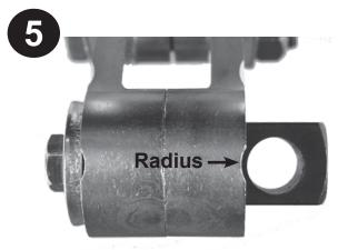
Slide handle clamp assembly into toggle and orient hole in lever clamp with radius in toggle.
