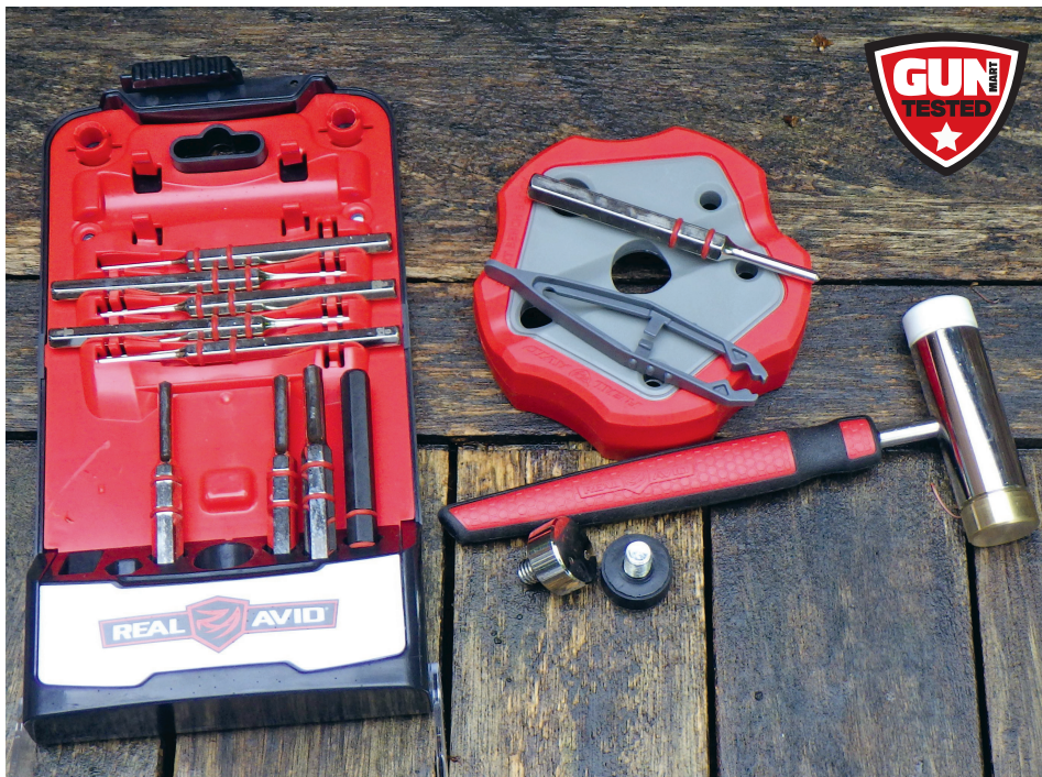
A great quality punch set complete with hammer, plus the smart bench block from Real Avid
