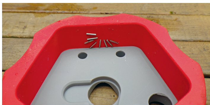
No more lost pins, thanks to the very smart magnet in the base of the bench block
