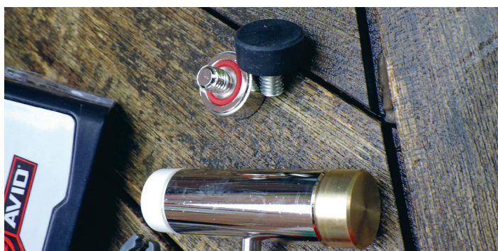
Interchangeable heads on the hammer ensure nothing gets damaged or marred
